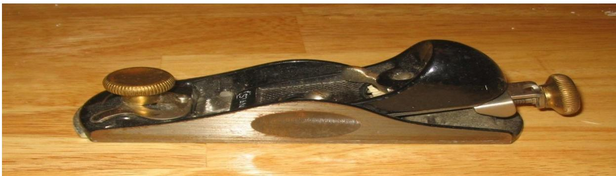
**USE:** It is used to smoothen rough surface of a wood.
