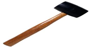
**USE:** It is used to drive wooden handled chisel.
