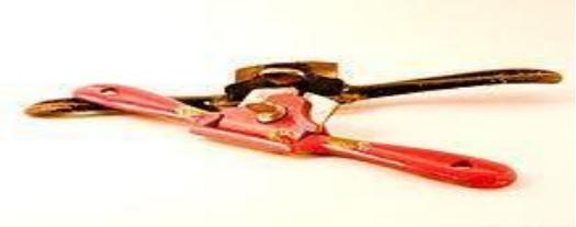
**USE:** It is used to shape wooden rods, for example, wheel spokes and chair legs.
