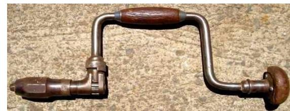
**USE:** It is used to drill holes in wood.
